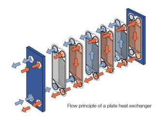
leakage to the surroundings will take place as gaskets around the edges of the plates seal the unit. The corrugation of the plates provides a suitable passage between the plates, support of each plate against the adjacent one and a strong turbulence resulting in maximum heat transfer efficiency.
